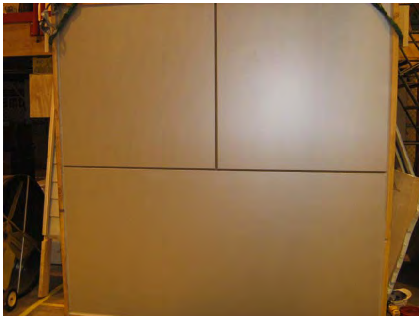
Photo No. 1 ACM Panel System (Dry Gasket)
